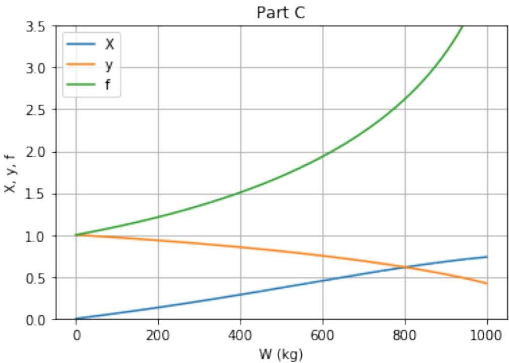
Reactor reaches a conversion of  $X = 70\%$  at  $W = 932.2674246272811 \text{ kg}$
