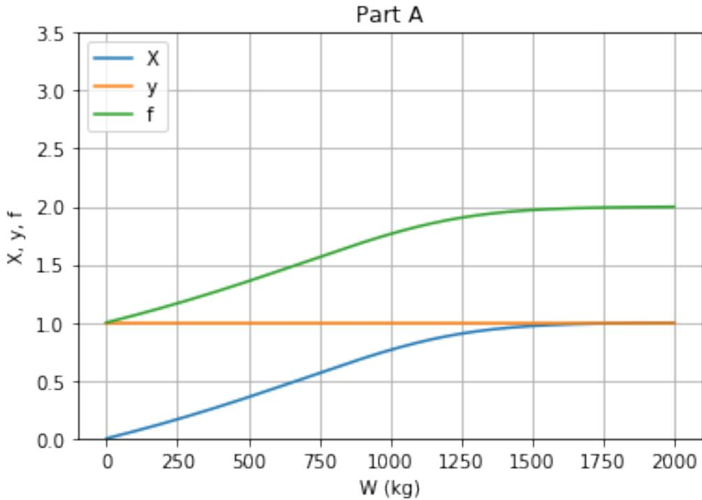
Reactor reaches a conversion of  $X = 80\%$  at  $W = 1054.1518509611706 \text{ kg}$
