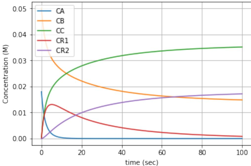
At 120 degrees Celsius, the Maximum effluent Concentration of R1 is 0.0131 M and the Flowrate is 0.017 M
